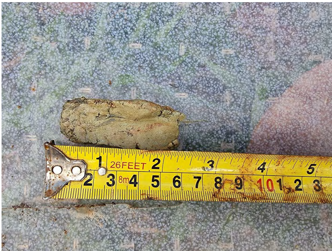
Ribbon test performed were consistent with Class 5 Soils - plastic bolus, slight resistance to shearing, medium size sand grains visible in finer matrix, 50-55 mm ribbon
